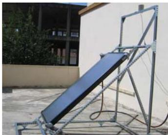
Photo 4. Rig and a Solar Collector during Testing Procedures
